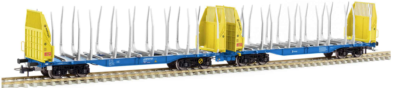
S657004 CD Cargo articulated double timber transport wagon Sgmrms | CD Cargo Doppel Holztransportwagen Sgmrms - A-IF 35 81 4657 004-1
