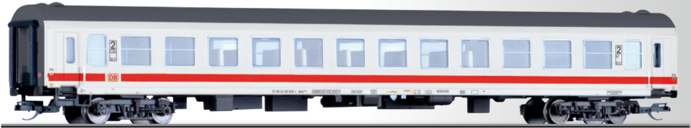
Reisezugwagen 2. Klasse Bimz 259, Bauart Halberstadt, der DB AG 2nd class passenger coach Bimz 259, type Halberstadt, of the DB AG
