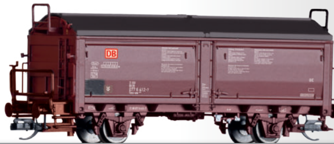
Schiebedach-/Schiebewandwagen Tims 858 der DB AG Sliding roof/sliding wall car Tims 858 of the DB AG
