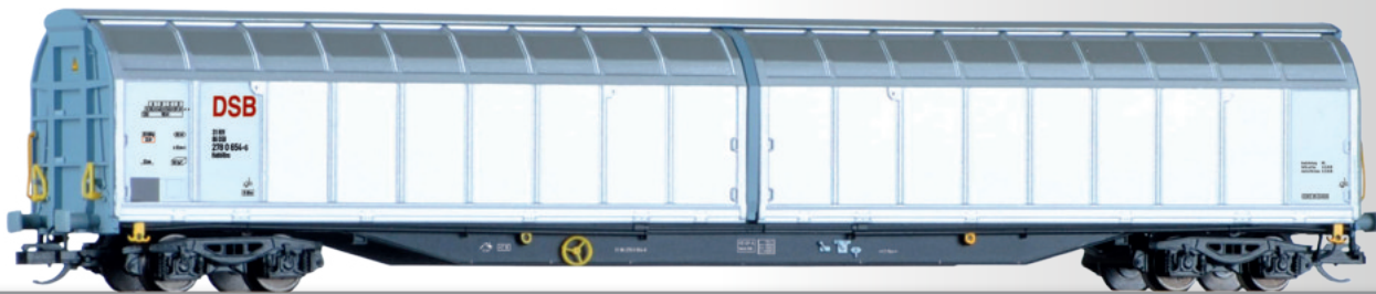
Schiebewandwagen Habbillns der DSB Sliding cover box car Habbillns of the DSB
