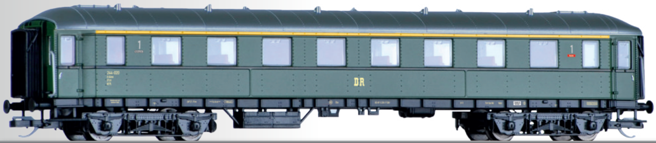
Reisezugwagen 1. Klasse A4ü der DR 1st class passenger coach A4ü of the DR
