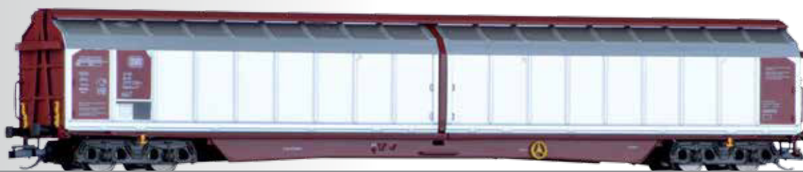
Schiebewandwagen Habbikks-tt 346 der DB Sliding wall box car Habbikks-tt 346 of the DB
