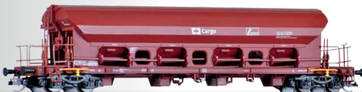
Schwenkdachwagen Tadgnss der ČD Cargo Swing roof car Tadgnss of the ČD Cargo
