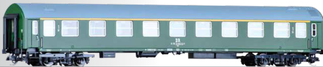
Reisezugwagen 1. Klasse Ame, Typ B, der DR 1st class passenger coach Ame, type B, of the DR
