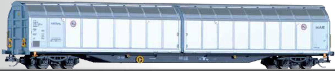
Schiebewandwagen Habbillns der Railion NL Sliding cover box car Habbillns of the Railion NL
