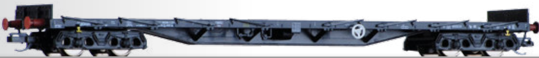
Rungenwagen Rs der PKP Cargo Stake car Rs of the PKP Cargo
