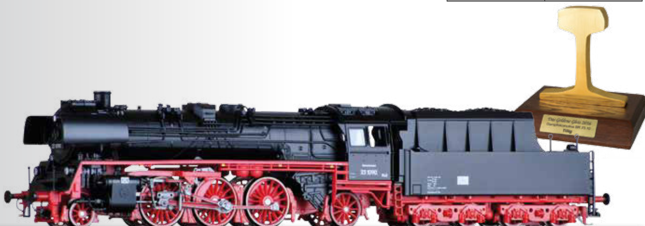
Dampflokomotive BR 23.10 der DR Steam locomotive class 23.10 of the DR
