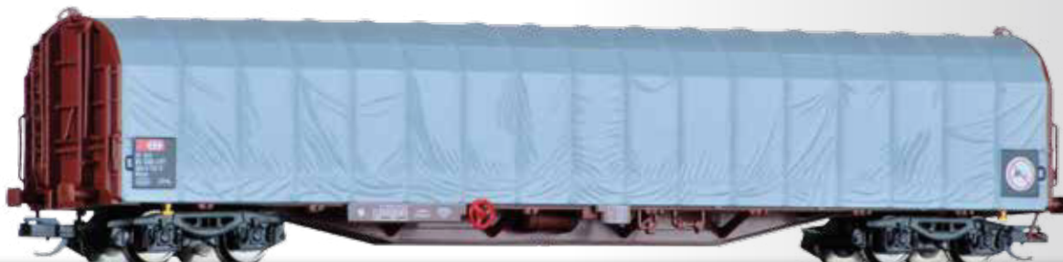
Schiebeplanwagen Rilns der SBB Sliding cover box car Rilns of the SBB
