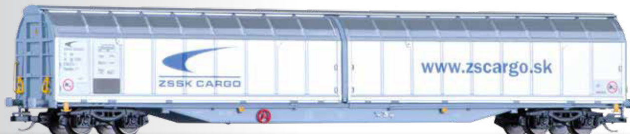
Schiebewandwagen Habbillns der ZSSK Cargo Sliding cover box car Habbillns of the ZSSK Cargo
