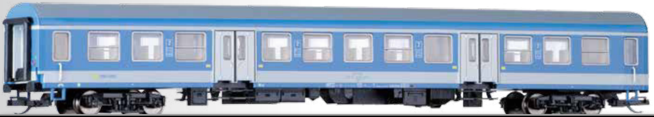
Reisezugwagen 2. Klasse By der MAV-Start 2nd class passenger coach By of the MAV-Start
