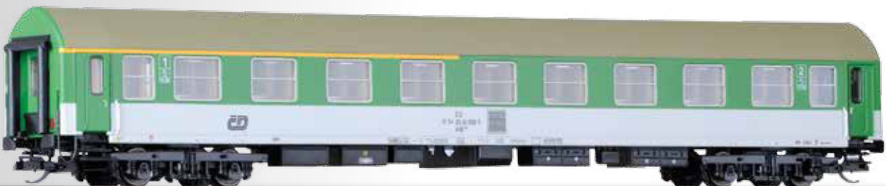
Reisezugwagen 1./2. Klasse, Typ Y/B 70, der ČD 1st/2nd class passenger coach, type Y/B 70, of the ČD
