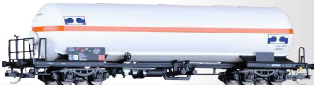
Gaskesselwagen Zagkks der Transgaz S.A. Gas tank car Zagkks of the Transgaz S.A.
