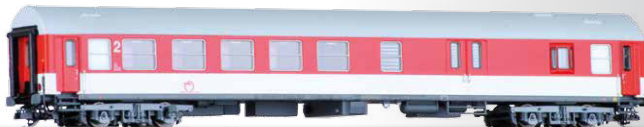
Sitz-/Gepäckwagen 2. Klasse, Typ Y/B 70, der ZSSK 2nd class passenger coach, type Y/B 70, with baggage compartment of the ZSSK
