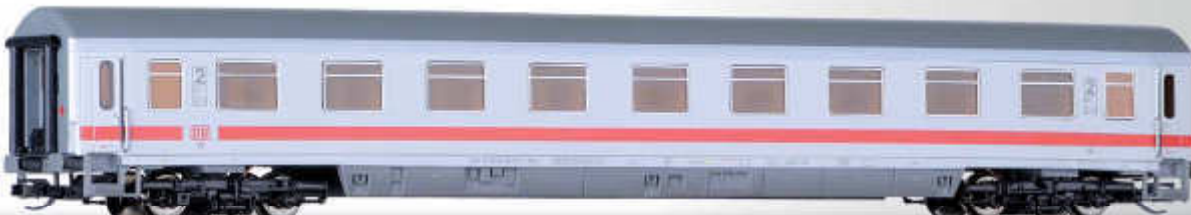
Reisezugwagen 2. Klasse, Bvmz 111.2 der DB AG 2nd class passenger coach, Bvmz 111.2 of the DB AG
