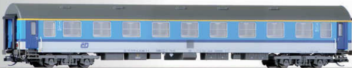
Reisezugwagen 1. Klasse, Typ Y/B 70, der ČD 1st class passenger coach, type Y/B 70, of the ČD
