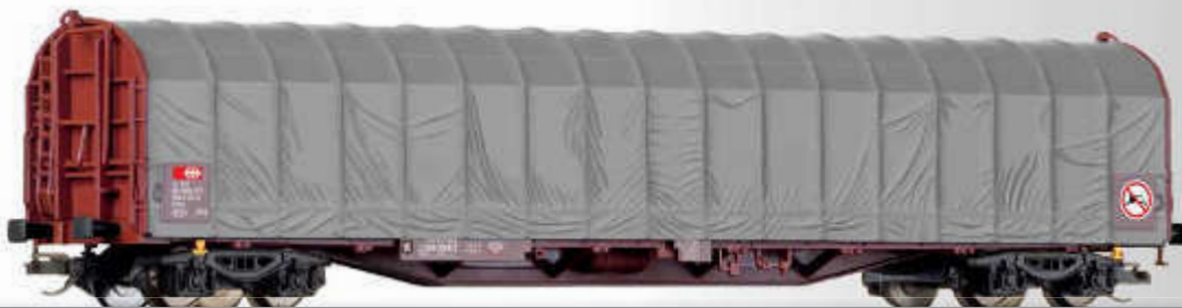
Schiebeplanwagen Rilns der SBB Sliding cover box car Rilns of the SBB
