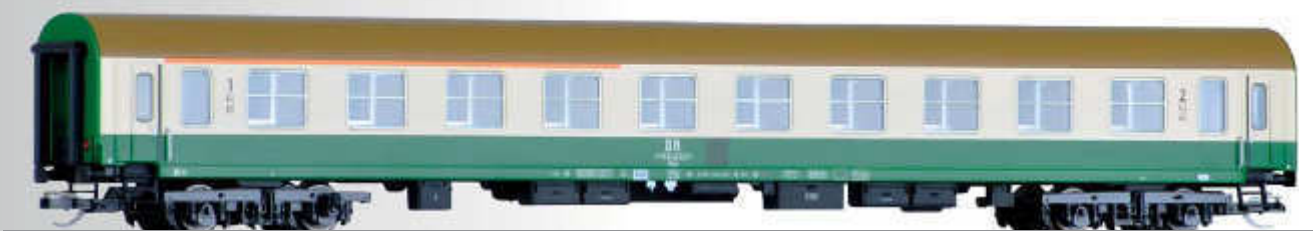
Reisezugwagen 1./2. Klasse ABm, Bauart Halberstadt, der DR 1st/2nd class passenger coach ABm, type Halberstadt, of the DR
