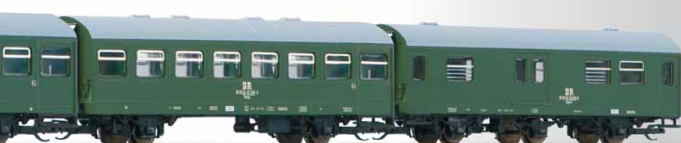
Passenger coach set of the DR with four different coaches (Bage, Bagtre, Baage, baggage car)
