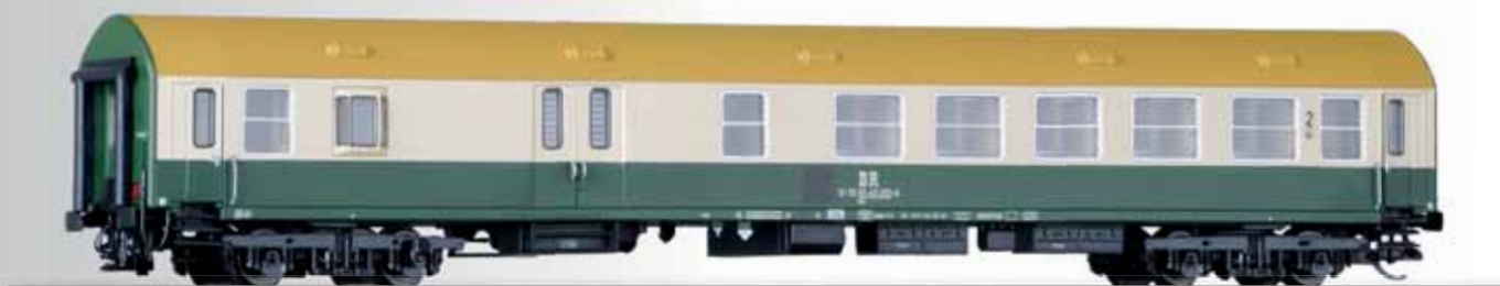
Sitz-/Gepäckwagen 2. Klasse, Typ Y/B 70, der DR 2nd class passenger coach with baggage compartment, type Y/B 70, of the DR
