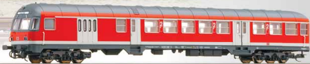
Steuerwagen Bnrdfz 463 der DB AG Driving cab coach Bnrdfz 463 of the DB AG
