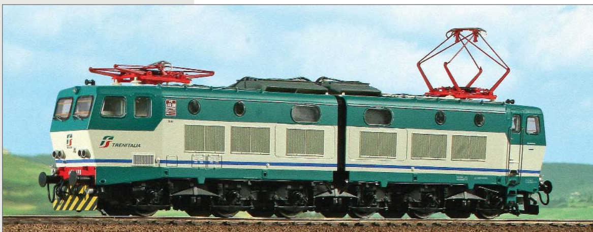
Locomotiva articolata delle FS E.656.598 (sesta serie). Livrea XMPR, pantografi Tipo FS 52, respingenti tondi. E.656.598 Italian Railways locomotive (sixth series). XMPR livery, Type 52 pantographs, round buffers. E-Lok E.656.598 der italienischen Eisenbahnen (sechste Bauserie). XMPR Lackierung, Typ 52 Stromabnehmer, runde Puffer.
