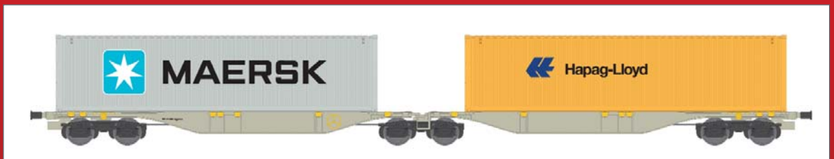
Carro intermodale Tipo Sggmrss 90 bimodulo Rail Cargo Austria con carico di container. Container wagon Type Sggmrss 90 Rail Cargo Austria, loaded with containers. Containerwagen Typ Sggmrss 90 Doppelmodul der Rail Cargo Austria, mit Containern.
