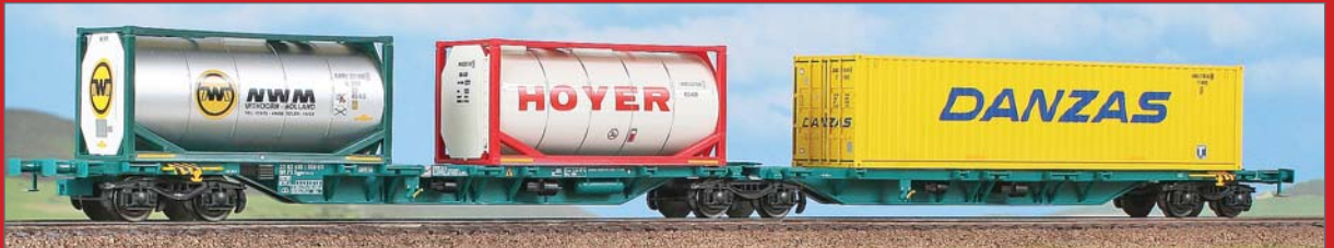
Carro intermodale Tipo Sggmrss con livrea verde della CEMAT con carico. Container wagon Type Sggmrss owned by CEMAT, loaded, green livery. Containerwagen Typ Sggmrss in der CEMAT, in grüner Lackierung, mit Containern.
