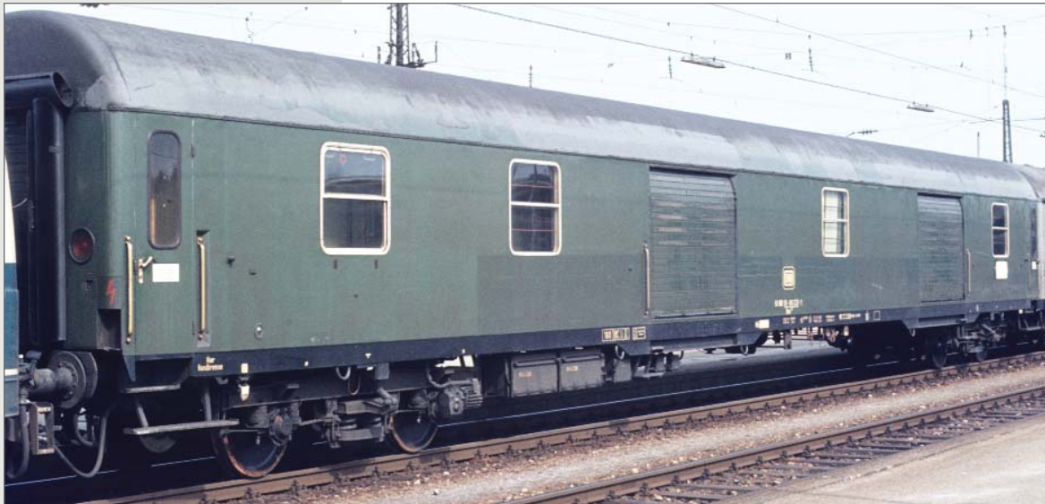
Bagagliaio Dums in livrea verde di origine con quattro porte. Dums baggage car, original green livery, four doors. Dums Gepäckwagen, original grüne Lackierung, vier Türen.
