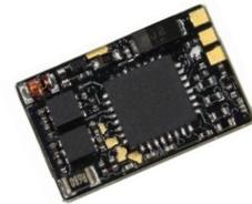
For Plug and Play you can use our **decoder item no. 66039** (train-O-matic). The decoder is completely programmed to use all functions of this modell (*excepting sound*).
